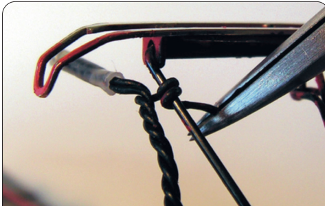
Halte draht am oberen Pantographen-Holm verdrehen. Twist the upper holding wire around the pantograph.
